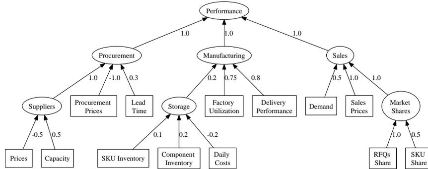
**Fig. 2.** A representational TAC SCM MRG. The **Performance** of the agent is divided into **Sales**, **Manufacturing** and **Procurement**, the three basic modules of a TAC SCM agent. Environmental impact is imported into the model with the nodes **Demand** and **Suppliers**
